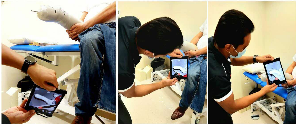
Technician performing a 3D scan of a transtibial amputee's stump using a handheld scanner
