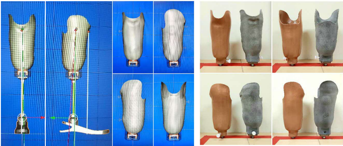
Left: 3D scan rectification and digital bench alignment. Right: Side-by-side comparison of a laminate socket (left) produced through conventional methods and a 3D printed socket (right) produced through the remote-digital method.
